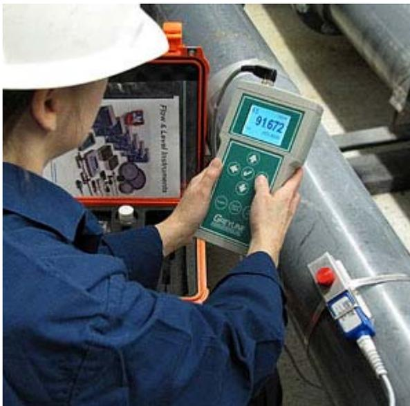
Ultrasound is sound generated above the human hearing range - above 20 kHz. Both Doppler and Transit Time flowmeter technologies are called "ultrasonic" because they operate far above the frequencies or sound range that we can hear.
